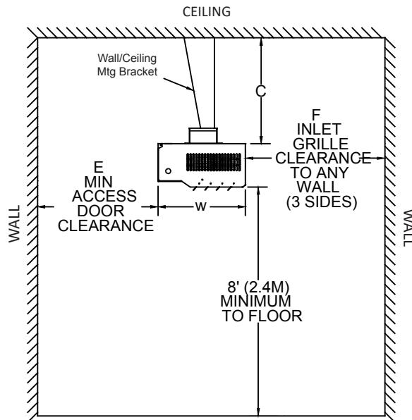
FIG. 4 VERTICAL CEILING MOUNT WITH MTG ARM
