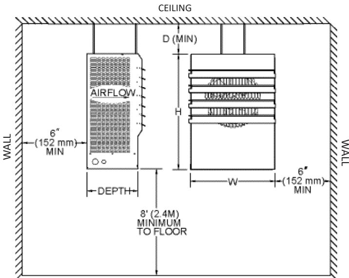
FIG. 3 HORIZONTAL CEILING MOUNT WITH THREADED ROD
