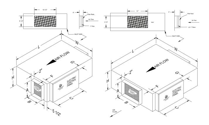
Control panel access right hand (U6L4) is standard as shown. For panel on opposite side access specify left hand (U4L6).
