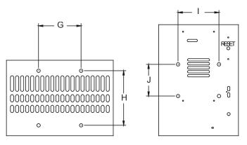
FIG. 5 THREADED ROD (3/8 - 16) ATTACHMENT POINT DIMENSIONS
