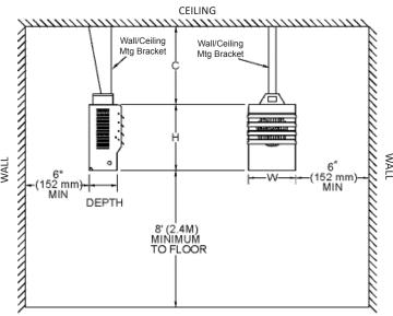
FIG. 1 HORIZONTAL WALL MOUNTING WITH MOUNTING ARM
