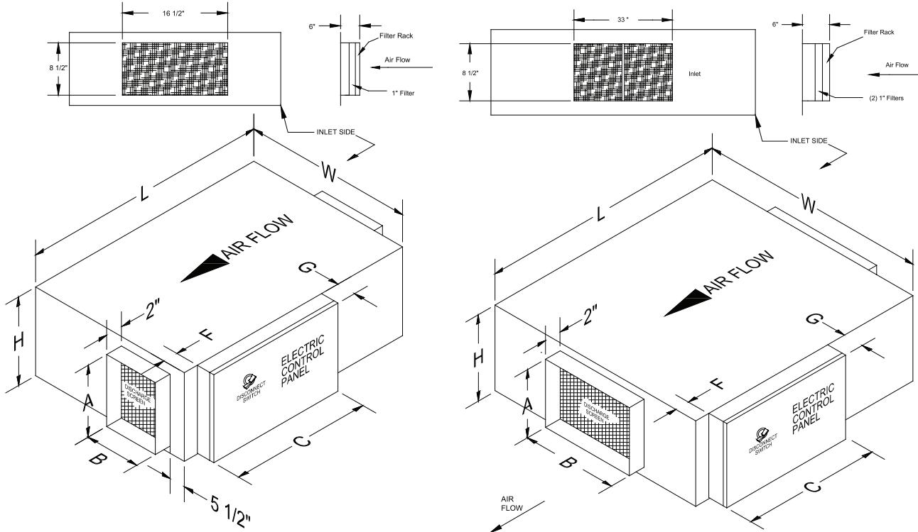
Control panel access right hand (U6L4) is standard as shown. For panel on opposite side access specify left hand (U4L6).
