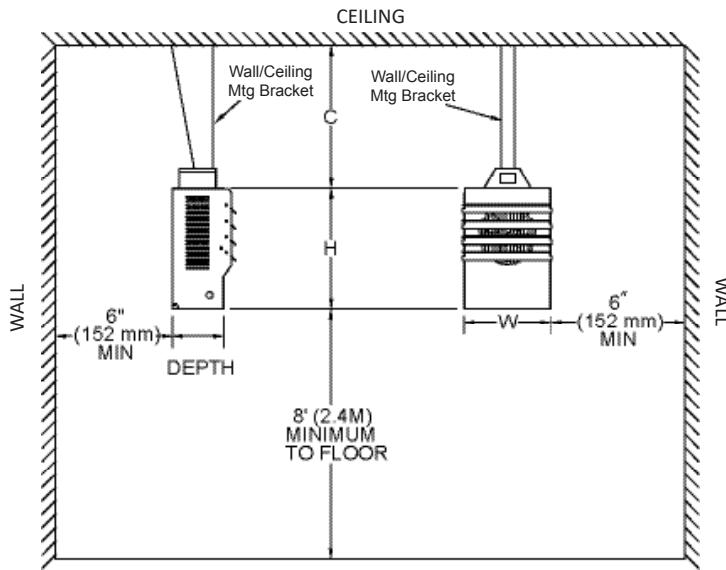
FIG. 2 HORIZONTAL CEILING MOUNT WITH MTG ARM
