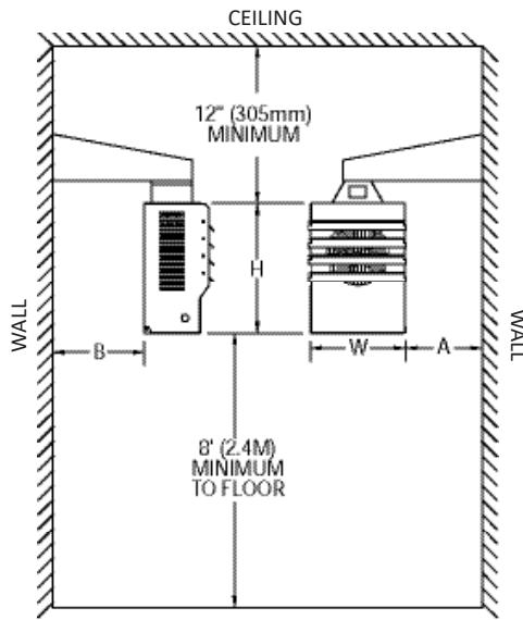
FIG. 1 HORIZONTAL WALL MOUNTING WITH MOUNTING ARM
