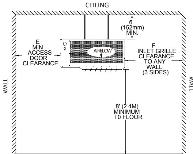
FIG. 6 VERTICAL CEILING MOUNT WITH THREADED ROD
