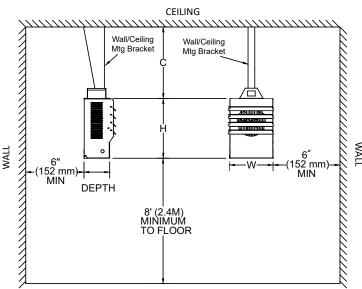
FIG. 1 HORIZONTAL WALL MOUNTING WITH MOUNTING ARM
