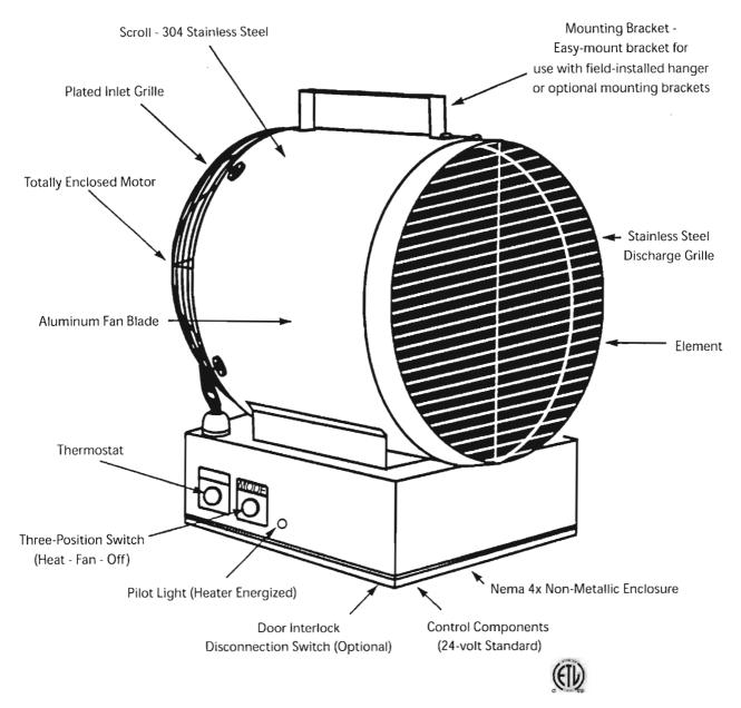
Rugged construction, stainless steel enclosure for use in wet\* and corrosive\* atmospheres (non-hazardous locations).
