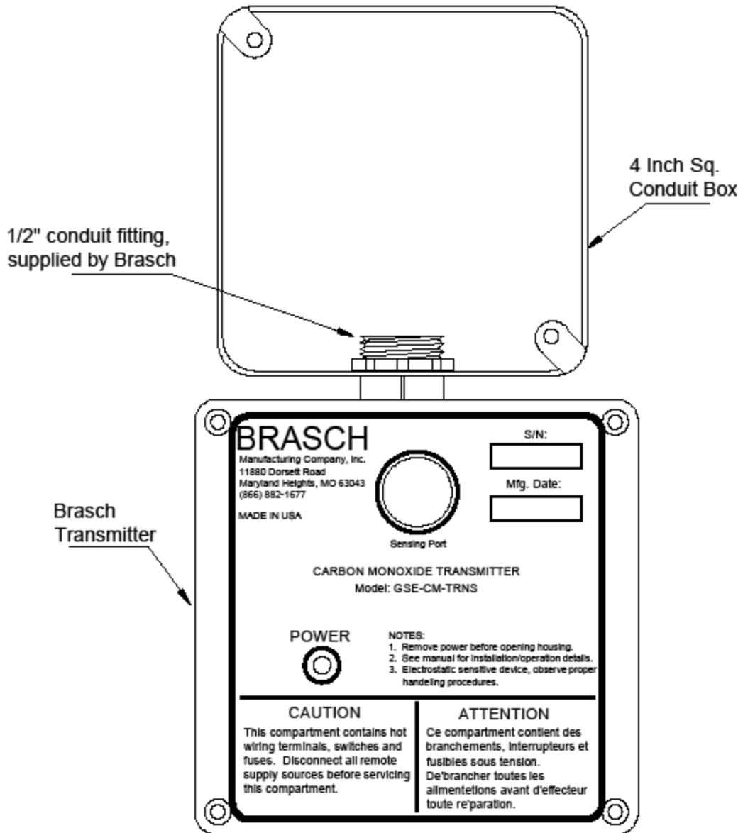
Fig. 6: Transmitter Mounting Method Using Four Inch Conduit Box
