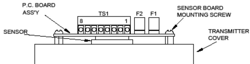
Fig. 1: Assembly View: Sensor P.C. Board to Transmitter Cover
