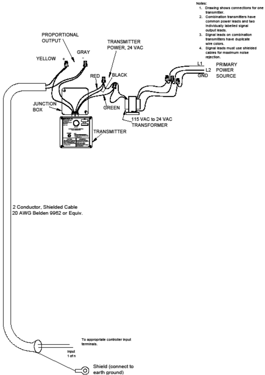
Fig. 2: Wiring Diagram, Others BMS to Remote Transmitter
